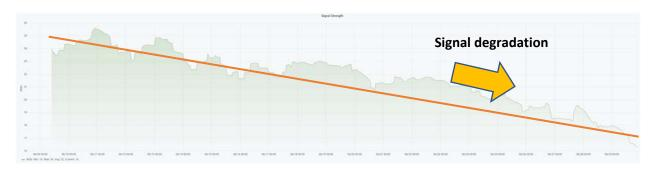
We found that raising the antenna higher above the vegetation can boost the radio signals dramatically. See this example below. Initially, the device had spotty communication. But, after adding the antenna extension, the radio signal doubled, while the antenna is still kept below the pivot hardware.
